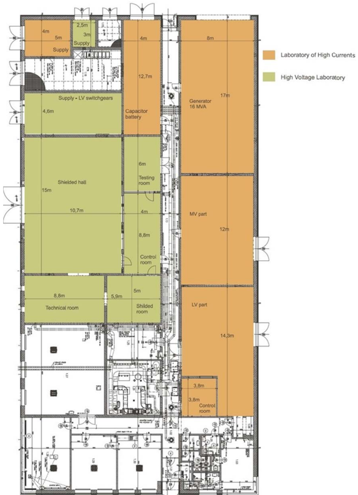
Fig. 7 Ground plan of CVVOZEPowerLab building
